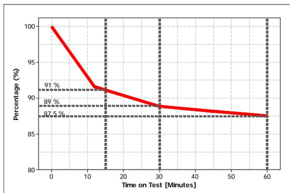
Figure 2: Example Survivor Curve Using VLF Withstand Data
