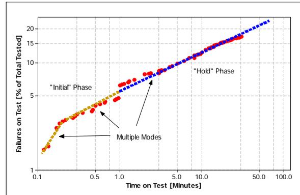
Figure 6: Weibull Plot of “Initial” and “Hold” Phase Failures on Test as a Function of Test Time
