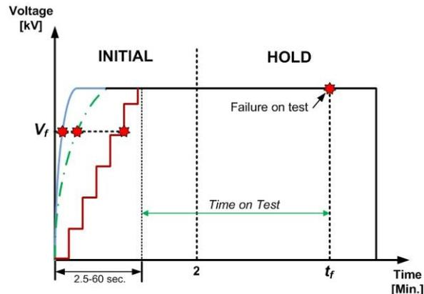
Figure 1: Withstand Test “Initial” and “Hold” Phases
