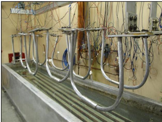
**Figure 1: ANSI C119.4 Current Cycle Submersion Test (CCST) for 750 kcmil Connectors**
