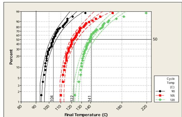
**Figure 6: Maximum Connector Temperatures by Cycle Temperature Conductor (750 kcmil Conductor)**
