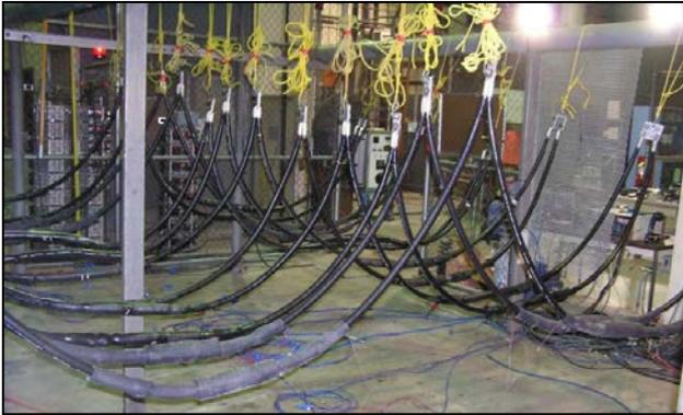
**Figure 3: IEEE 404 Style Load Cycle Test for Complete Joints on 1/0 AWG Conductor Cable**
