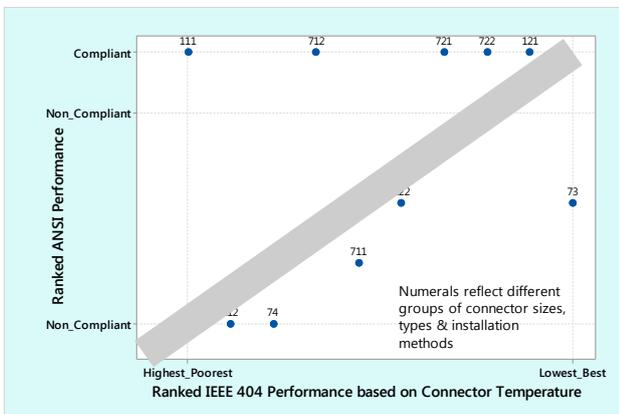
**Figure 7: Correlation of Rank Order from IEEE 404 Style Tests and ANSI Tests**
