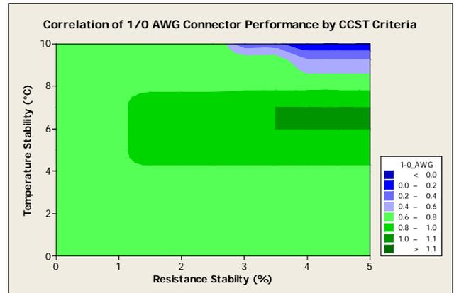
**Figure 8: Test Correlation Plot for 1/0 AWG Conductor**
