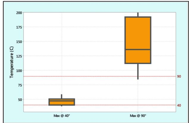
**Figure 4: Maximum Temperatures Achieved by 1/0 AWG Connectors Inside Joints at 40 and 90 °C in a Box and Whisker Format**
