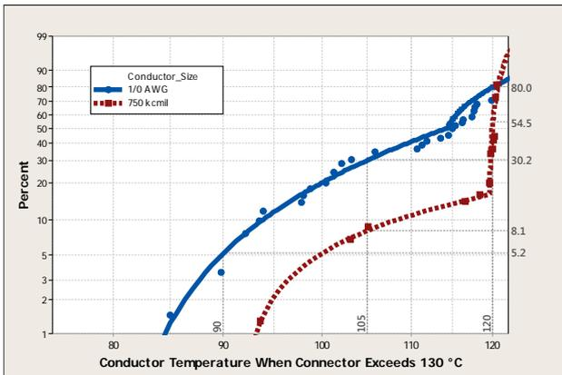
**Figure 5: Conductor Temperatures when the Connector within the Joint exceeded 130 °C (multiple Weibull distributions)**
