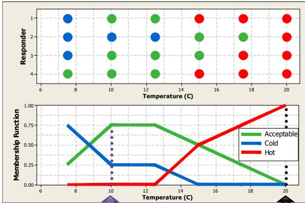
Figure 2: Example conversion of diverse responder input to Fuzzy Logic Membership Functions
