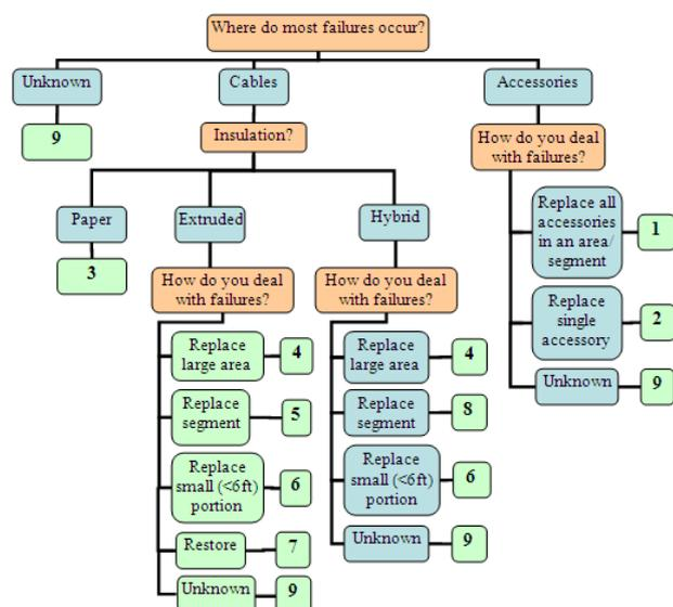
**Figure 1: Example of a simplified Asset Management flowchart for selection of Diagnostic Techniques**
