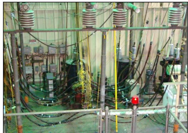
Figure 7: IEEE 404 Style Load Cycle Test
