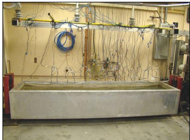
**Figure 1: ANSI C119.4 Test Setup – Current Cycle Submersion Test (CCST)**
