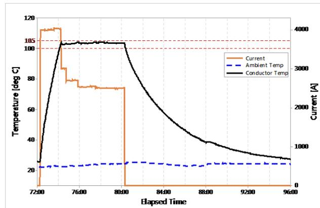
**Figure 1 Current / time recipe for the combined protocol (Table 2)**
