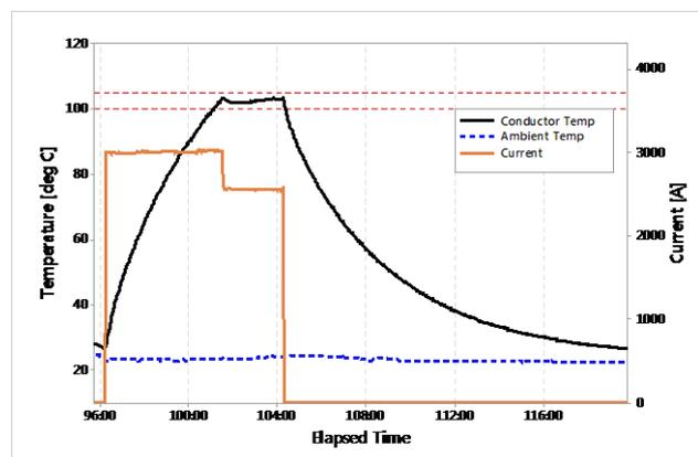
**Figure 2 Current / time recipe for the combined IEC / ICEA protocol**
