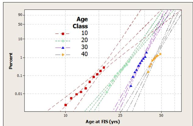
**Figure 8: Age segregated Weibull Curves for failures in service**
