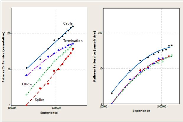
**Figure 6: Crow AMSAA Analysis of segregated failures (cable, elbow, splice & termination) for two different utility areas – left Area D & right Area N**
