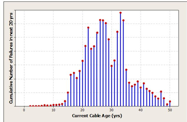
**Figure 10: Contributions to the failures in the next 20 years based on current cable age**
