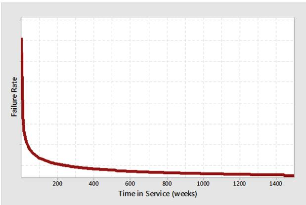
**Figure 2 Hazard Curve derived from Weibull Curve**
