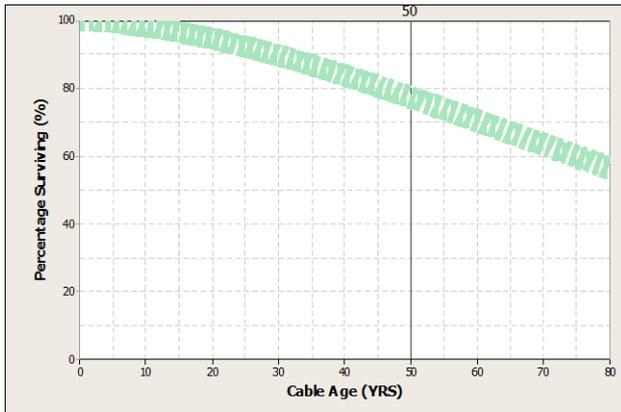
**Figure 9: Survivor Curve constructed from the four separate Weibull Curves shown in Figure 8**
