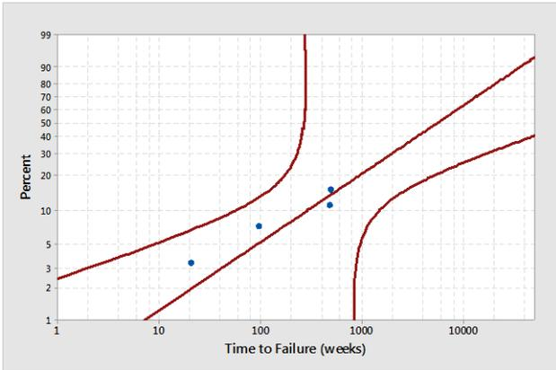
**Figure 1 Weibull Curve for time to failure in service**
