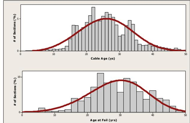
**Figure 7: Age Histogram of installed sections (derived from purchase records) – top and failing sections (derived from failure and installation records) - bottom**
