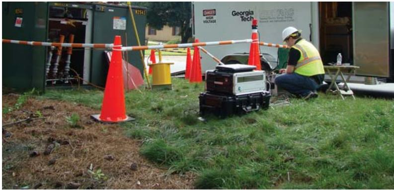
Working out of this test lab on wheels, NEETRAC Research Engineer Josh Perkel is performing diagnostic tests on a utility's underground cable circuit.
