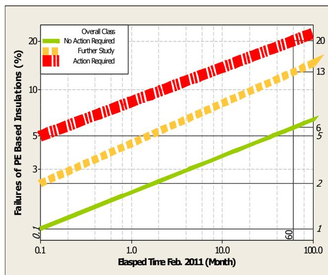
Figure 5. Diagnostic Performance Curves for Tan  $\delta$  Measurements on Cable Systems with PE-Based Insulations.
