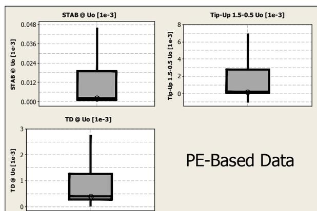
Figure 3. PE Based Cable Systems Dielectric Loss Feature Data in a Box and Whisker Format (the open symbol is the mean of the data).
