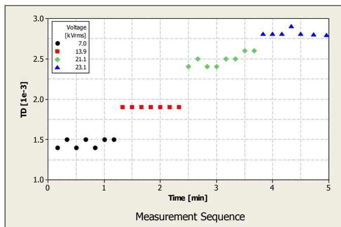
Figure 2. Measured Tan  $\delta$  data from a PE Cable System in Service (25 kv system operating at 13.9 kV).
