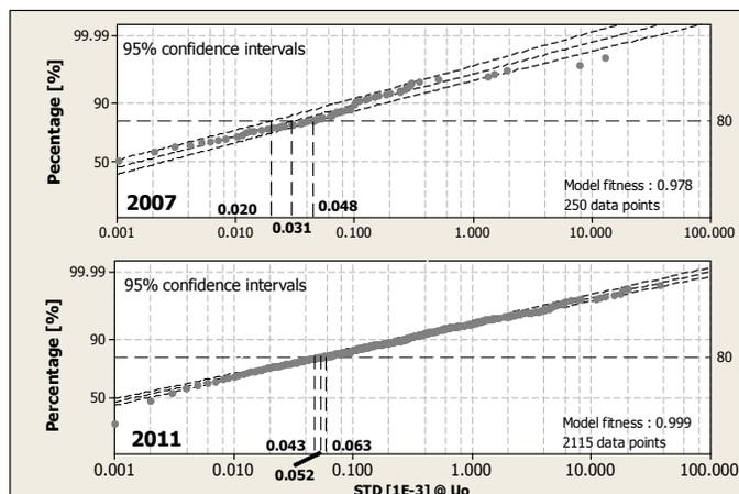
Figure 8. Comparison of 2007 (top) and 2011 (bottom) Probability Distribution Plots for Tan  $\delta$  Stability at  $U_0$  using Weibull Distributions with 95% Confidence Intervals.
