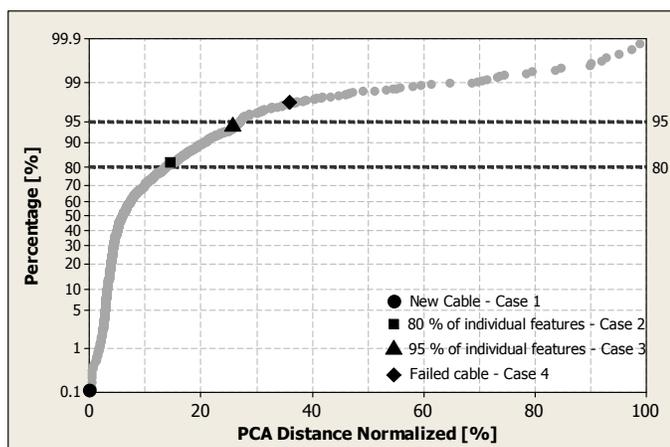
Figure 16. Empirical Cumulative Distribution for the Normalized PCA Distance for PE-Based Cable Systems.
