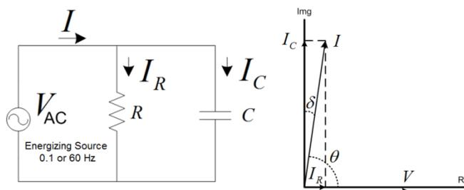
Figure 1. Equivalent Circuit for Tan  $\delta$  Measurement and Phasor Diagram.
