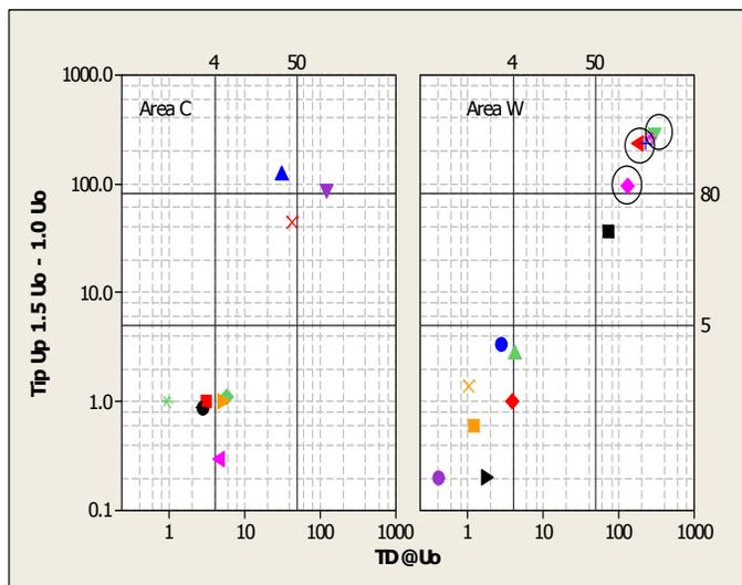
Figure 6. Tan  $\delta$  Results from 2007 Testing – Open Symbols Indicate Failures in Service in 2010-2011.
