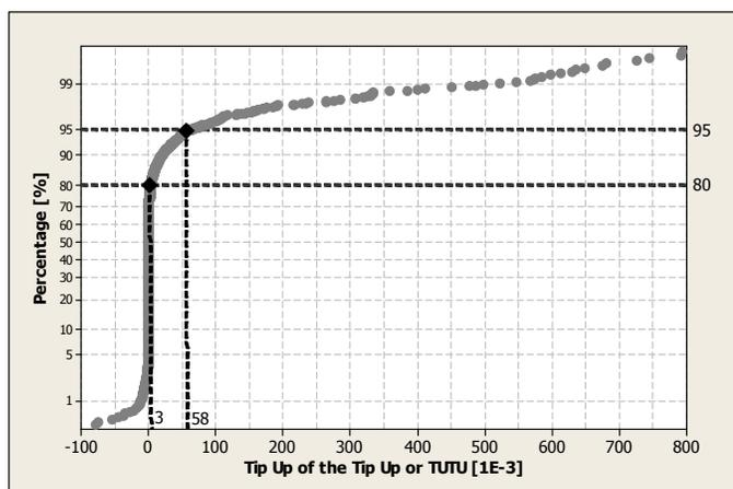
Figure 13. Cumulative Distribution Function for TUTU for PE Based Insulation.
