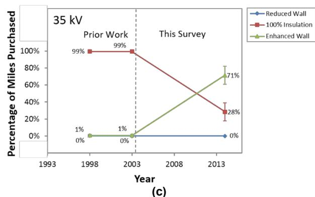
**Figure 4: A Fifteen-Year Trend in Purchased Cable Length by Insulation Thickness.**
