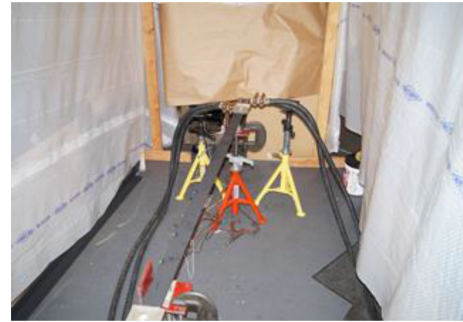
Fig. 4. Draft free enclosure for natural convection experiments.
