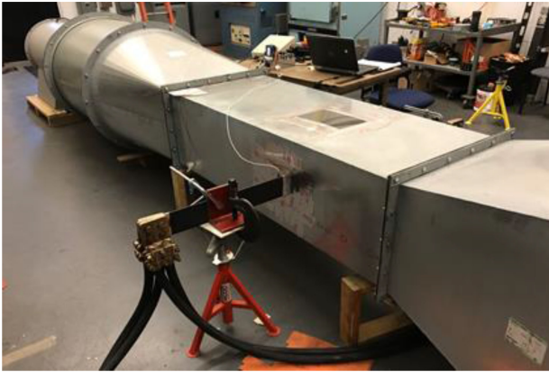
Fig. 2. Wind tunnel for forced convection experiments.
