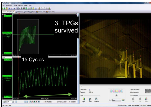
Figure 3: Example Waveform and High Speed Video for 0.089 m (3.5 in) Spacing
