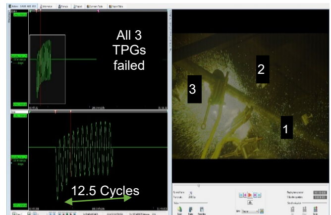
Figure 2: Example Waveform and High Speed Video for 0.305 m (12 in) Spacing
