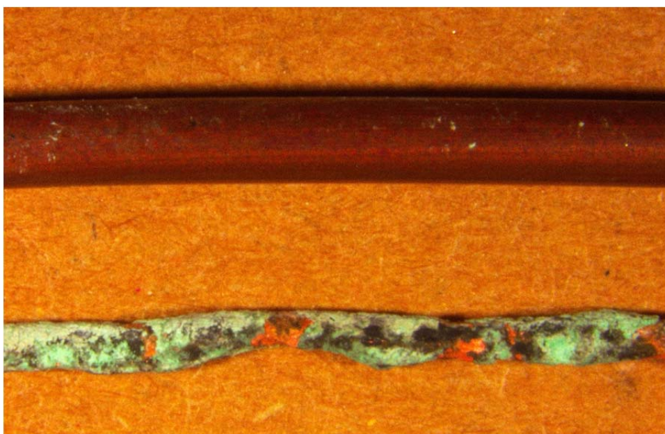
Figure 2: Corrosion of Concentric Neutral Wire Resulting in Loss of Metallic Shield Cross Sectional Area and Contact with Cable Insulation Shield (#14 AWG)
