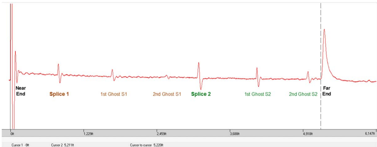
Figure 21: Splice and Ghost Reflections as seen in a TDR Unit from Field Tests of a 25 kV XLPE Cable System with Two Splices (TDR pulse of 100 ns) (See Case 5 in Table 6)
