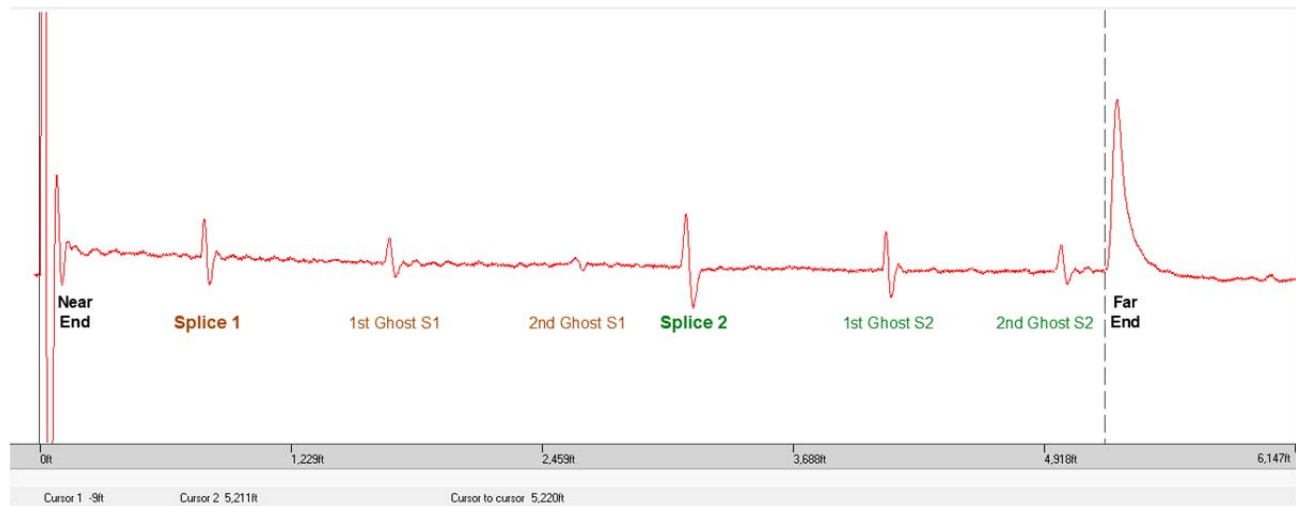
Figure 24: Splice and Ghost Reflections as seen in a TDR Unit from Field Tests of a 25 kV XLPE Cable System with Two Splices (TDR pulse of 100 ns)
