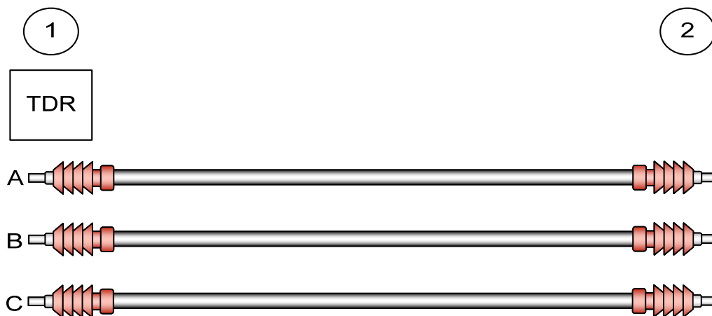
Figure 5: Three-Phase Section under Test Using TDR
