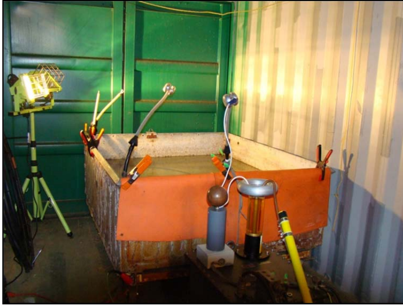
Figure 69: Test Set-up with Water Tank, Transformer, and Capacitive Divider
