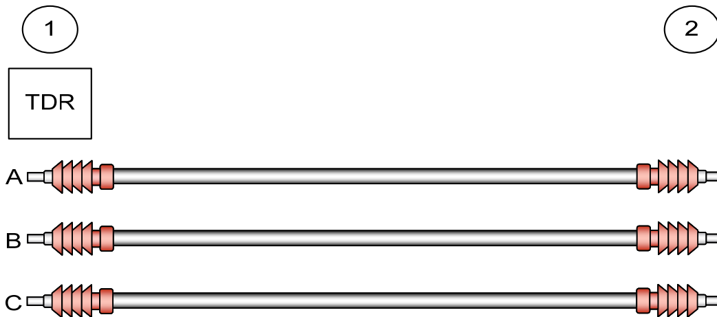
Figure 14: Three-Phase Section under Test Using TDR
