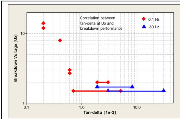
**Figure 4:** VLF breakdown strength versus average Tan  $\delta$  value for service aged cables measured in the laboratory.
