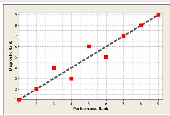
**Figure 5:** Performance Ranking plot for Tan  $\delta$  and breakdown strength for data from Figure 4.
