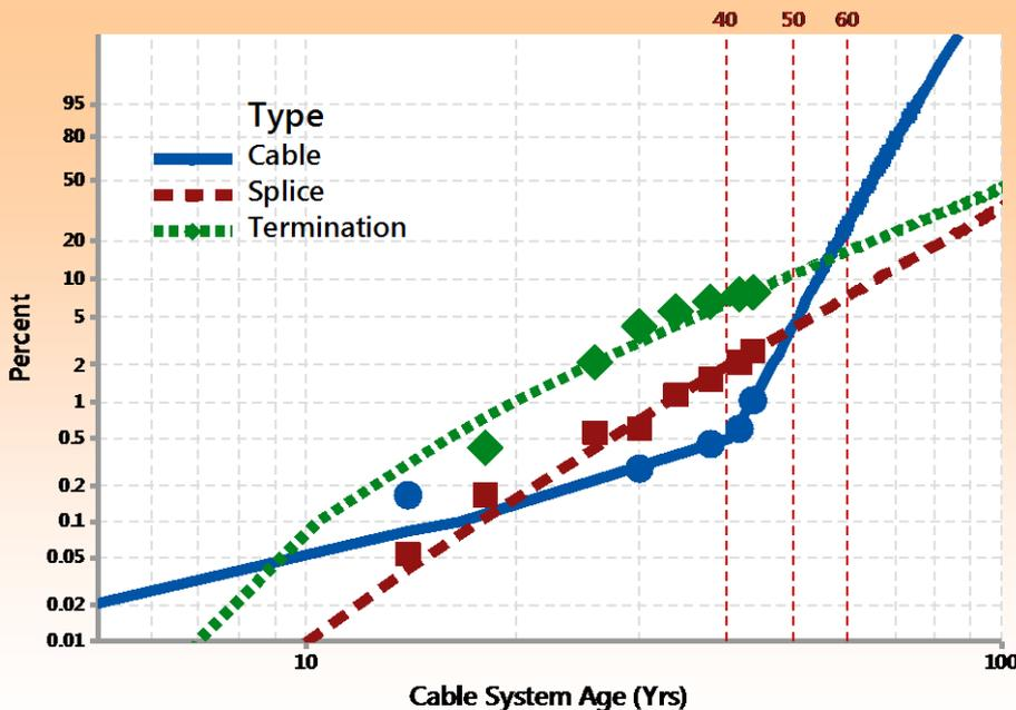
*For an XLPE cable system under normal operating conditions and moderate loading installed in ducts 95% of cables and splices will survive to age 50*
