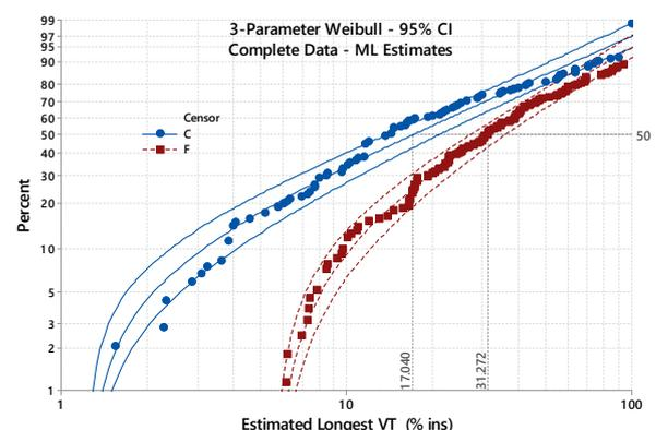
**Figure 6 Estimated longest vented trees - failure in service (F) and survival (C)**
