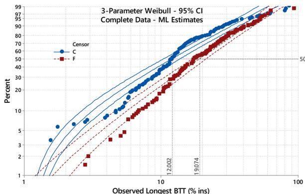
Figure 7 Distribution of longest bow tie trees, by fail in service (F) and condition assessment (C)
