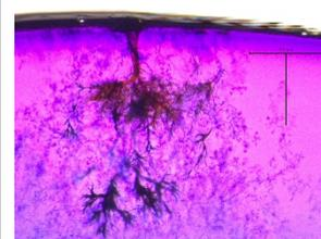
**Figure 4: vented tree growing from the insulation shield with some electrical treeing**
