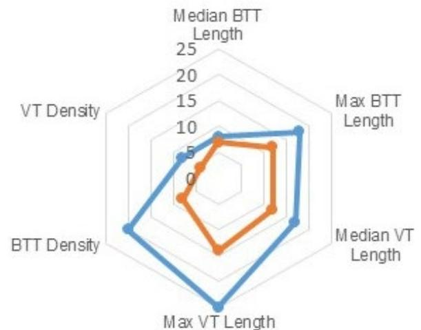
**Figure 9: Radar Plot of Descriptors for Failed (blue) and Condition Assessment (red) (all insulations)**
