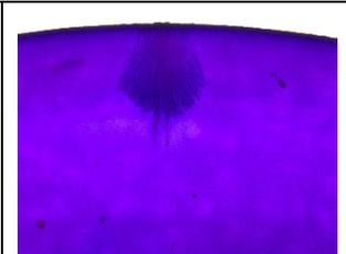
**Figure 3: vented tree growing from the insulation shield**
