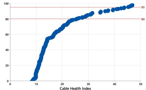
**Figure 10 Cumulative probability of the Cable Health Index (calc from principal components) for PE based insulations – low CHI’s represent good, high CHI’s represent poor health**
