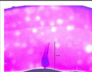
**Figure 2: vented tree from a protrusion on the conductor shield**
