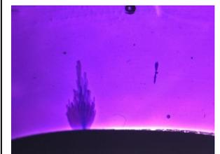
**Figure 5: vented tree growing from protrusion on conductor shield and bow tie tree growing in insulation**
