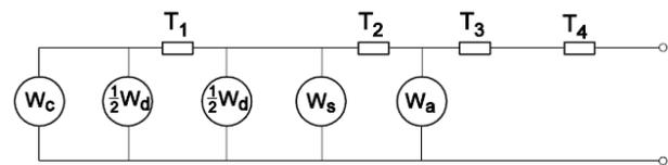
Figure 4: Ladder Network for Steady State Current or Temperature calculations (IEC60287-1-1)
