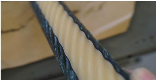
Figure 3: Cable Deformation Due to Elevated Temperature Operation
