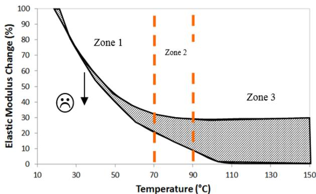
Figure 2: Polymeric Insulation Elastic Modulus
