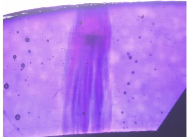
**Figure 4: Water Tree through 100% of Insulation**
